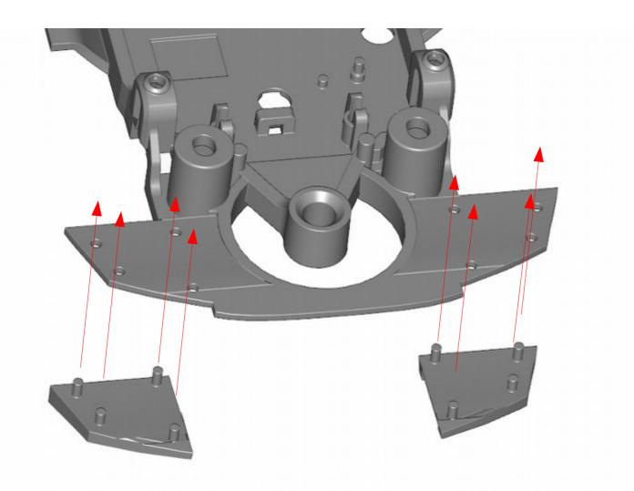
If you wondered what the small plastic parts under the base of the Skyline's box are for... We call them sliders: because of the shape of the chassis, which must follow as much as possible the original car's chassis, like most saloon cars the Skyline has a tendency to tip over. These little plastic pieces help counteract such tipping tendency.
