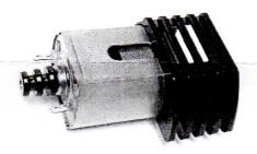
2. Slide heatsink on the motor from the pinion end.
