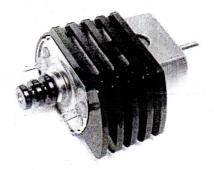
3. Slide heatsink all the way to the brush end of motor, and install motor in car!
