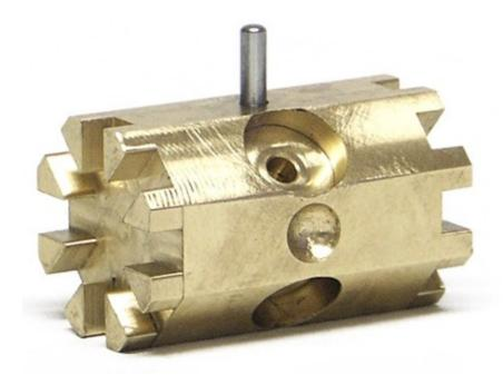
The multifunctional brass tool, depending on the operation to be performed, must be inserted in the main body with the plug downwards, in case of the extractor, or the pinion housing downwards, in case of the press. The pinion housing for this element were designed to house pinions with a diameter ranging from 5.5 mm to 7.5 mm without damaging them.
